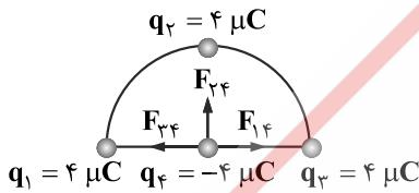
$$F_{24} = \frac{k |q_2||q_4|}{r_{24}^2} = 9 \times 10^9 \frac{4 \times 10^{-6} \times 4 \times 10^{-6}}{(2 \times 10^{-2})^2} = 36 \cdot j$$
