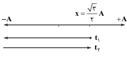
$$\begin{aligned} x &= A \cos\left(\frac{\pi}{T} t\right) \Rightarrow \frac{\sqrt{3}}{2} A = A \cos\left(\frac{\pi}{T} t_1\right) \\ &\Rightarrow \begin{cases} \frac{\pi}{T} t_1 = \frac{\pi}{6} \Rightarrow t_1 = \frac{T}{12} \\ \frac{\pi}{T} t_2 = \frac{11\pi}{6} \Rightarrow t_2 = \frac{11T}{12} \end{cases} \end{aligned}$$
