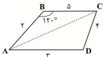
$$\left. \begin{aligned} AC^2 &= AB^2 + BC^2 - 2AB \times BC \cos 120^\circ \\ AC^2 &= AD^2 + DC^2 - 2AD \times DC \cos D \end{aligned} \right\} \Rightarrow 2^2 + 5^2 - 2 \times 2 \times 5 \cos 120^\circ = 2^2 + 4^2 - 2 \times 2 \times 4 \cos D$$
